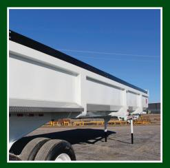
Three-Piece Tub Design Full-length sides and floor provides greater strength.
