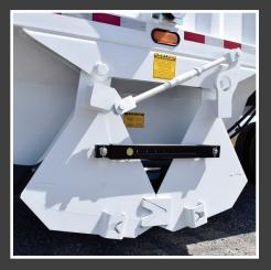
Pitch Control Link/Slide Lock Pin The Pitch Control Link adjustment is used to keep the doors closed. The Slide Lock Pin is designed to lock the doors while traveling, dumping and during repairs.
